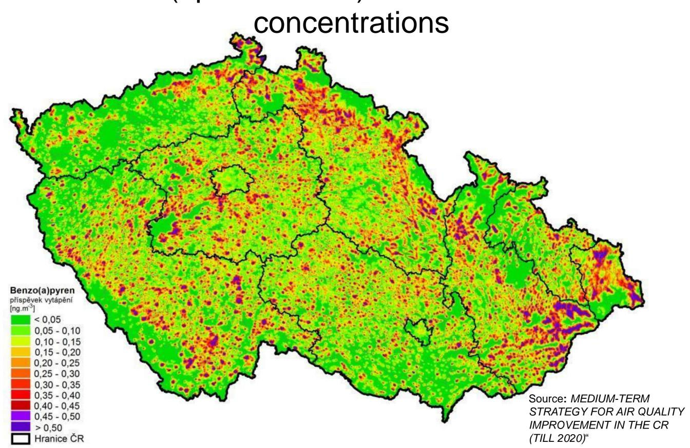
Contribution of small combustion stationary sources (up to 300 kW) to PM10 annual mean concentrations
